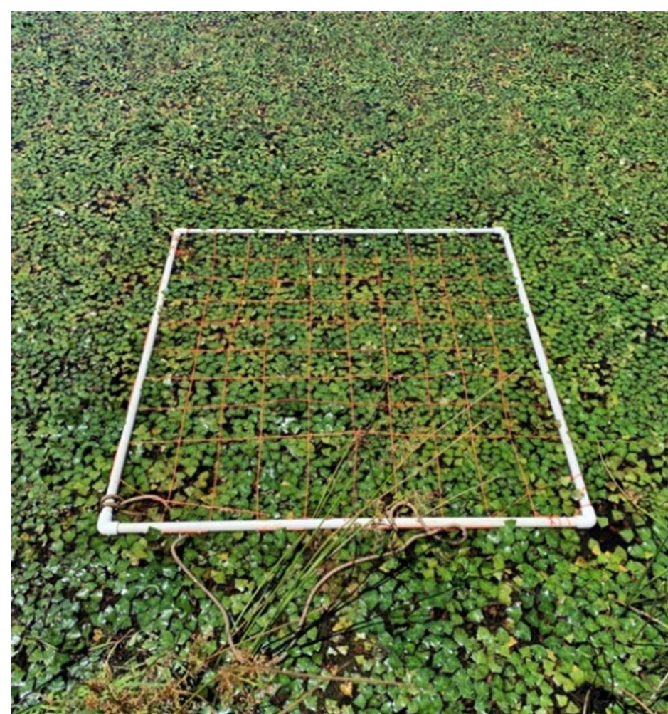
Fig. 2. Quadrat used for sampling T. bispinosa coverage (QC). Whole quadrat is 1 m x 1 m and is divided into 100 squares each 0.1 m x 0.1 m.
