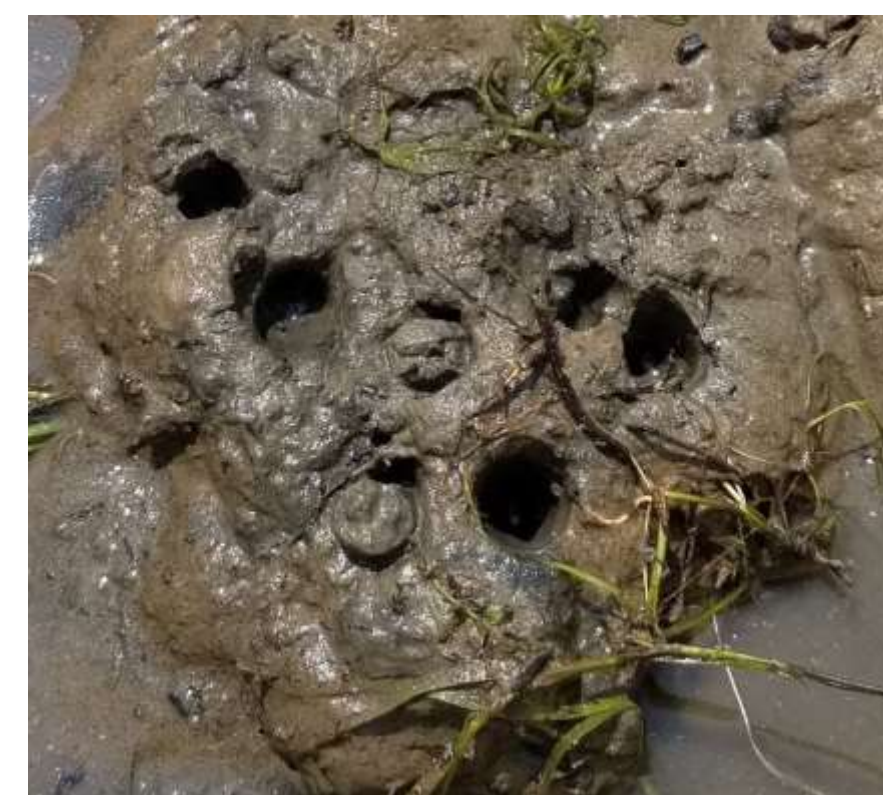
Ponar sample with individual subsamples obtained by cork borer
