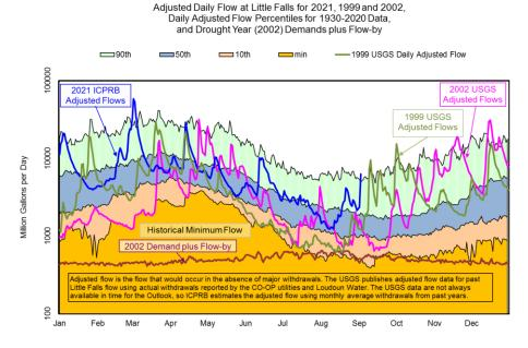
Little Falls flow statistics are based on 1930 through 2020 USGS published gage flow, "USGS 01646502 POTOMAC RIVER (ADJUSTED) NEAR WASH, DC". To create this flow record, the USGS has added historical water supply withdrawals from
