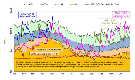
Little Falls flow statistics are based on 1930 through 2014 USGS published gage flow, "USGS 01646502 POTOMAC RIVER (ADJUSTED) NEAR WASH, DC". To create this flow record, the USGS has added historical water supply withdrawals from the Potomac as reported by FW, WSSC, the Aqueduct, and Rockville to the Little Falls gage flow record.
