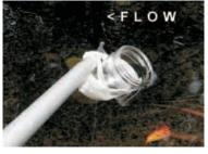
**DO** sample with the opening of the bottle facing upstream, into the flow so the water will enter directly into the bottle.
