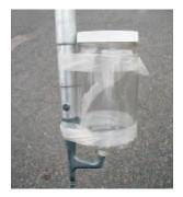
**DO** attach a bottle to a pole for sampling, if necessary. A boathook is used in this example, and the bottle is attached with filament strapping tape.
