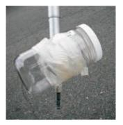
If the water is too shallow to sample with the bottle upright on the pole, try taping it on sideways, but tilted up slightly.
