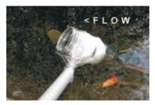
**DO NOT** sample with the bottle facing downstream, when using a pole or sampling by hand. Water flowing past your container, pole, or hand and into the container can be contaminated by such contact.
