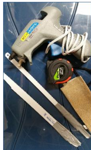
Above: Your primary cutting tool: a reciprocating saw blade with small teeth. Wind one end with duct tape for a handle. Retractable blade knives also work well.
