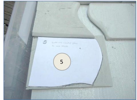
Pieces 3 and 5 overhang the base, because the bin bottom is narrower than its top. The small overhang is unlikely to break and prevents water from going down the side during use.
