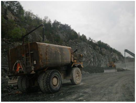
Quarry sump water truck used for dust control.
