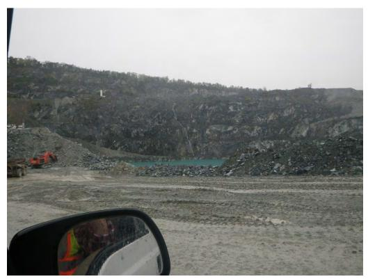
Active mining of SW highwall adjacent to quarry sump. Quarry discharge line is evident.
