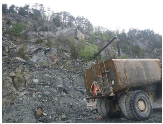
Typical blast damaged highwalls.
