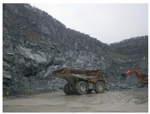
Active mining. High angle joints present in adjacent bench wall.
