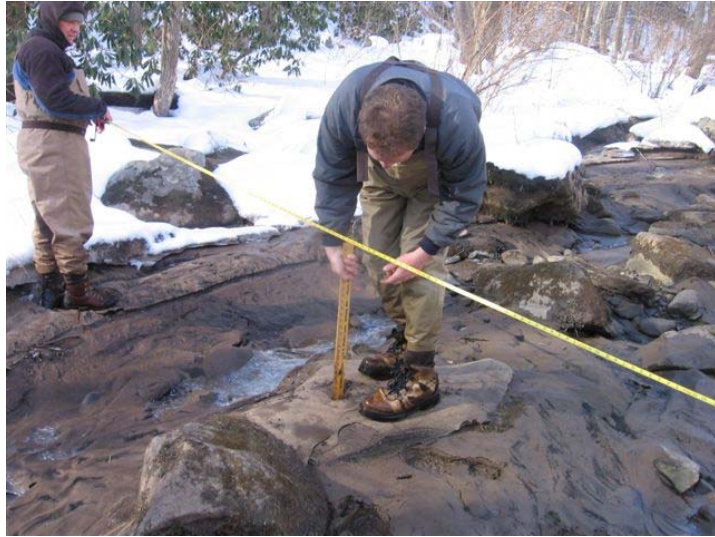
Figure 2 MD DNR Fisheries Biologist, Alan Klotz, measures the depth of fine sediment deposited in the Savage River.
